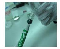
Fill ink into pen. And then, fill reducer with using other syringe.
