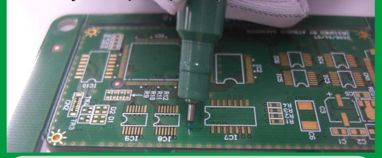
SKETT-PEN is innovative tool specialized for repairing solder mask defect of P.W.B.
