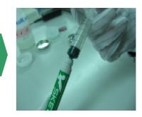
Fill ink to pen. And then, fill reducer with using other syringe.
